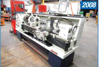
**BENIGN** Gap Bed Engine Lathe With 24" Swing, 86" Between Centers, 12" Chuck, 2,000 RPM, DRO, 3" Bore, s/n 0267 s/n 071
