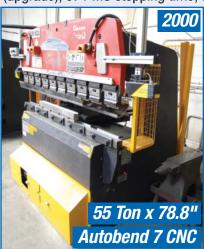
2000 **AMADA** RG-50 CNC Hydraulic Press Brake With 55 Ton X 78.8" Capacity, **HURCO** Autobend 7 CNC Control, 59.9" Between Capacity, 66.75" Between Housings, Housings, 3.94" Stroke, 14.58" Open Height, 15.75", 12" Open Height, Flat Die, s/n 114 15.75" Throat, SICK V4000 Light Curtains, 460V, 3 Phase s/n 509758
