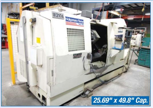
NAKAMURA-TOME TMC-35 CNC Lathe With FANUC CNC Control, 25.69" Swing, 49.8" Between Centers, 10 Station Turret, 10" Chuck, 2.52" Bar Cap., Tool Presetter, Chip Conveyor s/n 0119
