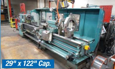
**TOS** SN71C/3000 Gap Bed Engine Lathe With 29" Swing, 122" Between Centers, 12" Chuck, 1,000 RPM, 3" Bore, DRO, 2 Steady Rests
