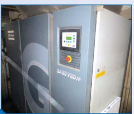
2007 **ATLAS COPCO** GA55VSD 75HP Rotary Screw Air Compressor With 18,366 Hrs., s/n AP1574461
