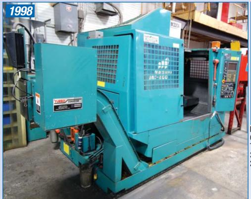
1998 MATSUURA MC-800VG CNC Vertical Machining Center With Yasnac CNC Control, 20" X 45" Table, Travels: X-31.5", Y-20", Z-20", Bt-40 Taper, 24 ATC, Chip Conveyor, 10/15 HP, 200/220 V, 3 Phase s/n 980313360
