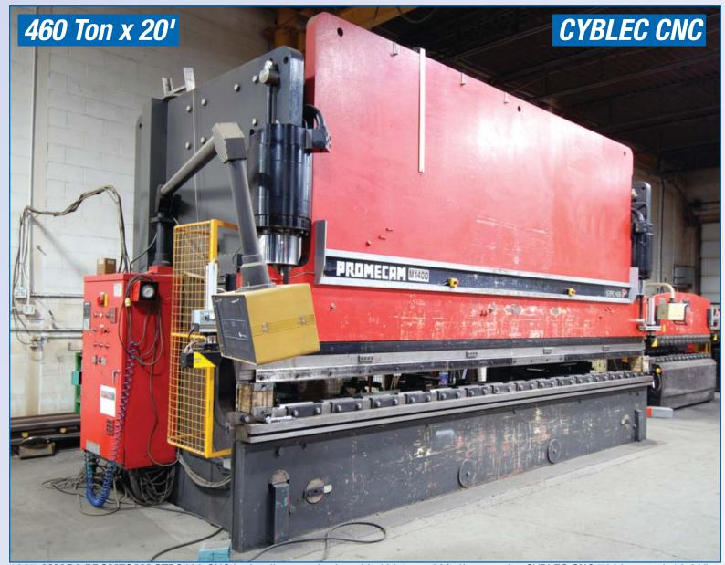
1987 AMADA PROMECAM STPC406 CNC hydraulic press brake with 460 ton x 20ft 4in capacity, CYBLEC CNC 7000 control, 12.60" stroke, 18ft 4" between housings, 25" throat (upgrade), 071 MS stopping time, SICK V4000 laser curtains s/n 60-0103
