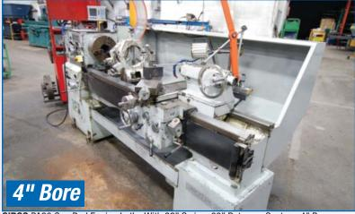
SIRCO PA20 Gap Bed Engine Lathe With 22" Swing, 68" Between Centers, 4" Bore, 1,500 RPM DRO
