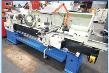
**TOS** SN 50 Gap Bed Engine Lathe With 21" Swing, 98" Between Centers, 16" Chuck, 2" Bore, DRO, 2,000 rpm, Steady Rests
