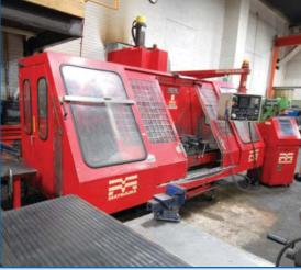
MATSUURA MC-1000VS CNC Vertical Machining Center With FANUC CNC Control, 19.5" X 55" Table, Travels: X-41.38", Y-19.63", Z-22", CAT 50, 35 ATC, 3600 RPM, 25 HP Spindle Motor (Rebuilt 2011) 220V, 3 Phase s/n 85024403
