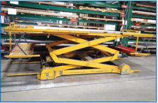
Motorized Track Mount Scissor Lift With 11ft 4" X 72" Lift Area
