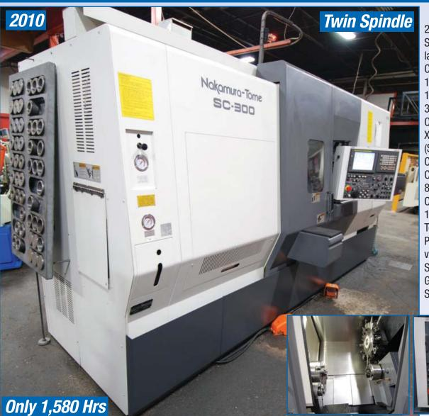
2010 NAKAMURA - TOME SC300 twin spindle CNC lathe with FANUC 18iB **CNC Control (Upgraded** 10.4" Color Screen), 13.78" Max Turning Dia., 31.89" Distance Between Opposed Spindles, Travels: X-8.76", Z-25", B-19.66" (Sub Spindle), 2.80" Bar Cap., 12" Main Spindle Chuck With 3,500 Rpm, 8" Opposed Sub Spindle Chuck With 3,500 Rpm, 12 Station Turret With Live Tooling, Tool Presetter, Parts Catcher, Chip Conveyor, KISAGE Coating On Slides, (Only 1,580 Hrs., Great Condition) s/n S311005
