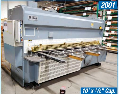
2001 **HACO** HSLX 3013, Hydraulic Shear With 10ft X 1/2" Cap., SC7 Front Operated Power Back Gauge, 39 1/4" Squaring Arm, Roller Supports, 575V s/n 69501
