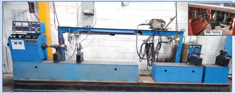
**DIA** CE 502 VS Electronic Dynamic Balancing Machine With 450 RPM For Shafts And 900 RPM For Propeller Shafts And Rotors, Weld Unit, Large Qty Of Attachments And Tooling s/n 10182
