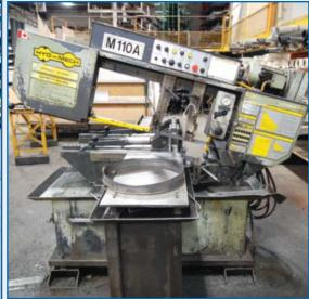
1991 **HYDMECH** S-20A Automatic Horizontal Bandsaw With 13" X 18" Capacity, 1-1/4" Blade, 5 HP Blade Drive Motor, 75-400 FPM, Clamping, s/n 10991558
