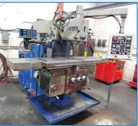
**TOS** Vertical Mill With 15.75" X 55" Table, 1,800 RPM, Power Feeds, With DRO
