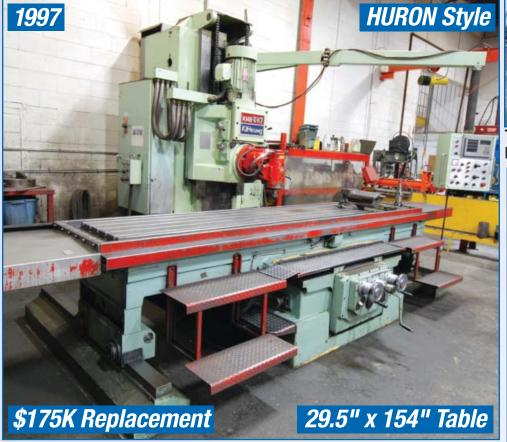
1997 **KIHEUG** KMB-U-H7 Universal Mill With HEIDENHAIN DRO, 29.5" x 154" Table, Travels: X-126", Y-39.37", Z-31.5", 8800Lbs Table load, Ball Screw XYZ, Weighs 33,000 Lbs, 50 Taper, Vertical Head, 18-1,300 RPM, 15HP, 220V 3 Phase s/n 7090501
