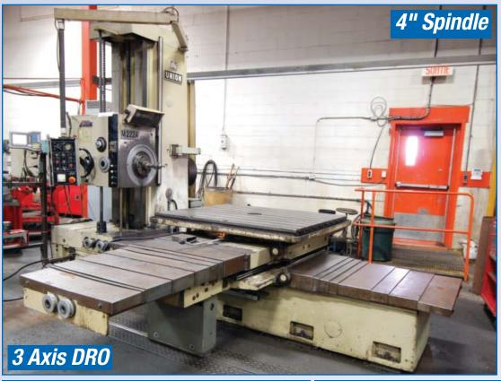
UNION BFT90-3 table Type Horizontal Boring Mill With 4" Spindle, 50 Taper, Facing Head, 55" X 49" Built In Rotary Table, Travels: X-63", Y-49", Z-63", 1,600 RPM, 15 HP, Facing Head, ACURITE DRO, Pendant Control s/n 0287
